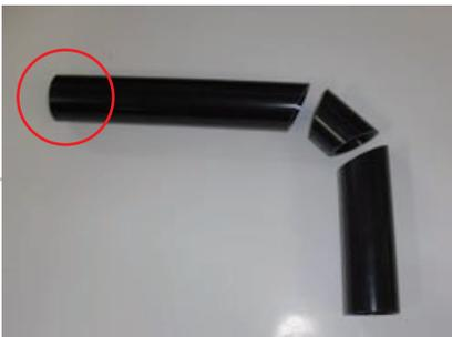
Make the inside of the pipe flared. Refer to the attached paper.
