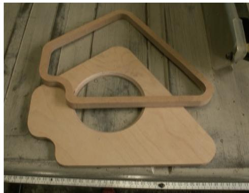
4. Stack the cut-out boards to make the side panel
