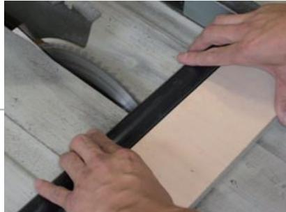
When you cut the pipe, apply wood piece to it for assistance.
