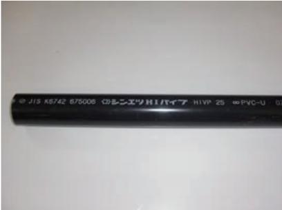
Use a PVC pipe. The inside diameter for front speaker: 25 mm, for subwoofer: 40 mm.
