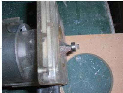
Use trimmer to slant the cut section.
