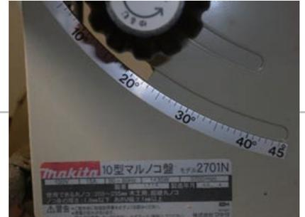
Adjust the degree of table saw at 22.5°.
