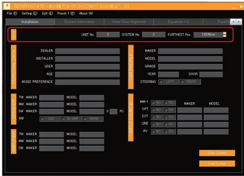
**UNIT No.** / Enter the number of the BEWITHSTATE connected. The main unit's Unit No. should be 1. In this manual, enter 1 into the Unit No. of the left channel and enter 2 into the Unit No. of the right channel.
