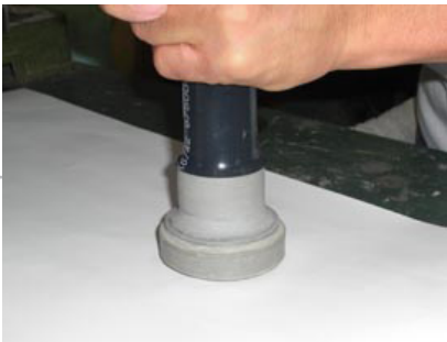
Stretch the heated edge.
