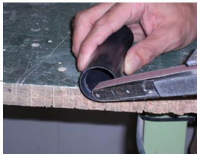
Use belt sander to make the slant part smooth.
