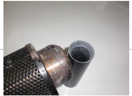
Heat the slant edge with heat gun or burner.
