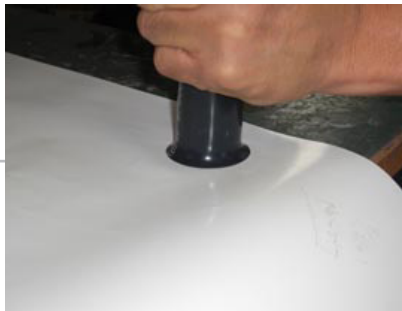
Stretch the heated edge.
