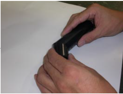
Glue both cut sections together.
