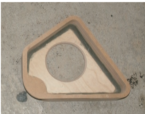
5. Apply putty to the corner of the back panel and the side panel and make it round and smooth
