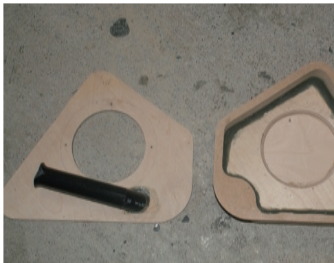
7. Fix the port onto the baffle board
