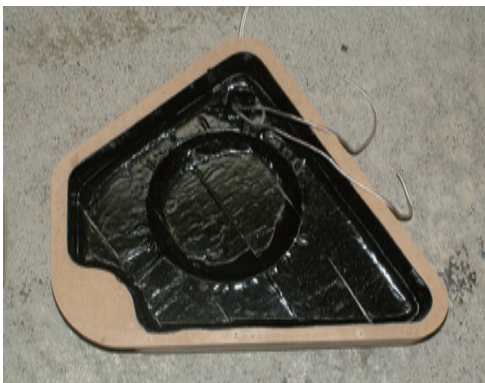
10. Apply butyl tape to the inside wall of the enclosure
