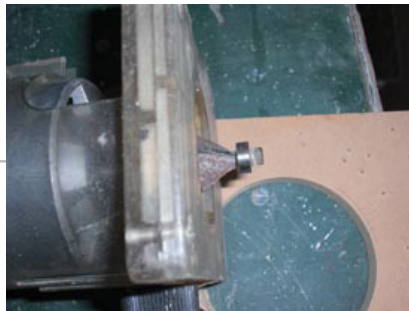
Use trimmer to slant the cut section.
