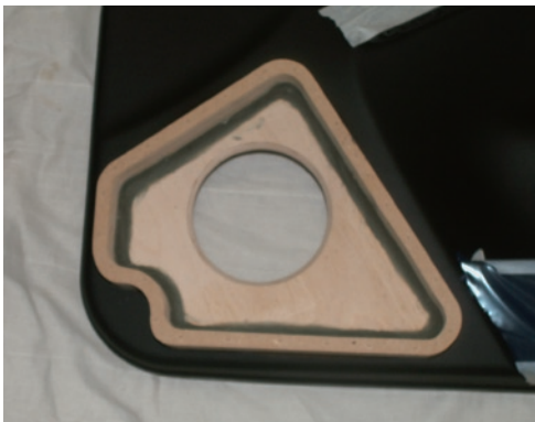
8. Make sure that the enclosure fits on the trim
