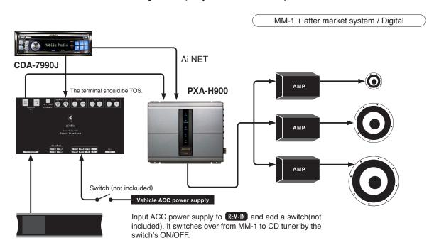
Note: The switch (not included) is necessary for switching over from MM-1 to another system (factory standard or after market system). Volume is controlled by CD tuner(7990J). Terminal of the digital cable(COAX) needs processing to fit on.
