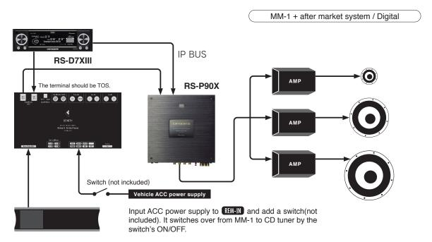
Note: The switch (not included) is necessary for switching over from MM-1 to another system (factory standard or after market system). Volume is controlled by CD tuner(RS-D7X). Terminal of the digital cable needs processing to fit on.
