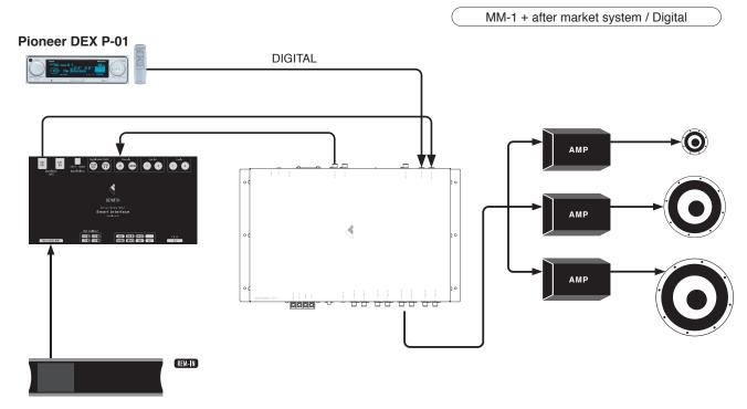
※ Terminal of the cable needs processing to fit on (for AZ-1 OPT2 input) With carrozzeria X serise, digital signal does not output from the head unit unless the processor is connected to IP BUS.
