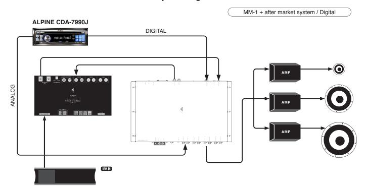
Digital output of ALPINE CDA-7990J is only for CD audio. The audio of the tuner should be inputted in ANALOG. The terminal of COAX input needs processing to fit on. The ANALOG input needs an adapter cable.
